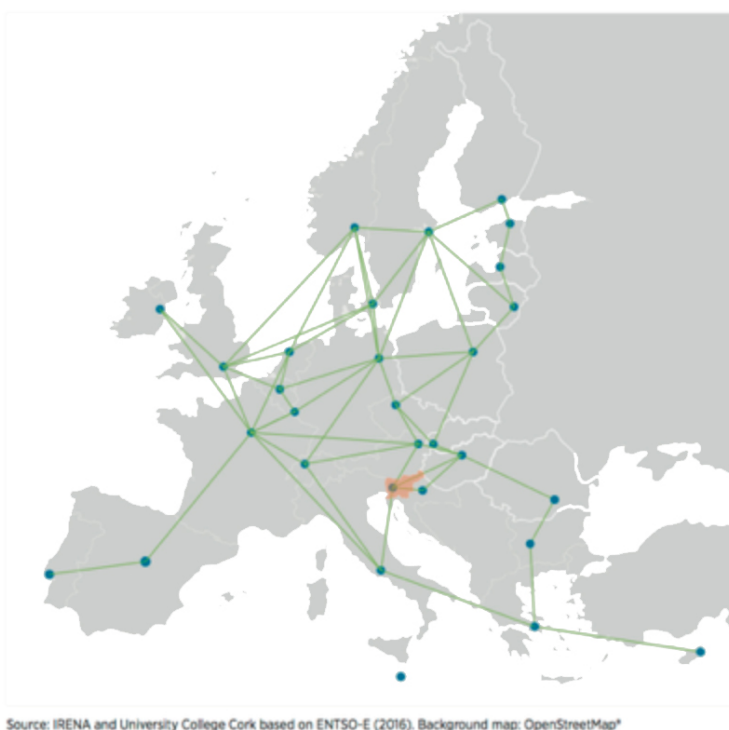
Figure 1 – Interconnections in the 2030 EU power system model 83
